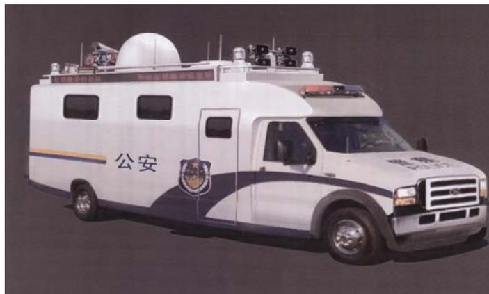
Fig1-1 A DZT2000A Mobile Satellite Earth Station
